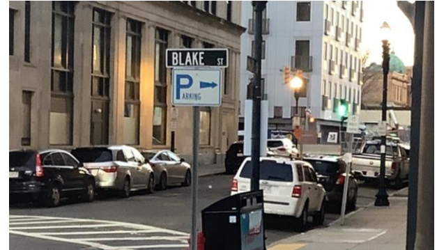
Scale of sign may be too small and lacks information. The placement of the sign is positioned after the intersection where the vehicle should be making a right turn.
