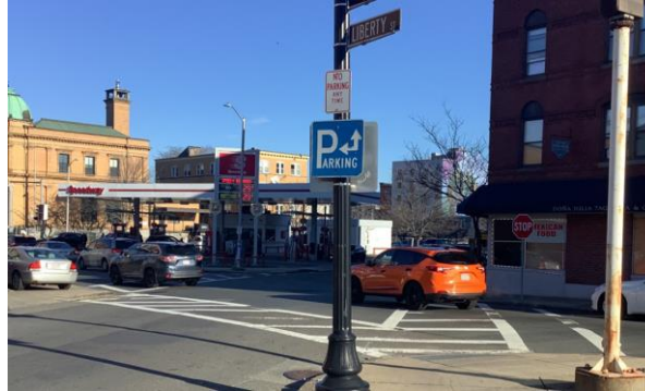
Parking sign is simple and legible but lacks information about the type of parking available (e.g., long vs. short-term). The placement of the sign is positioned at the intersection instead of ahead of the approach to allow drivers to reposition.
